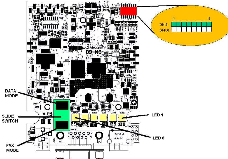
DIP switches are located on the top of the board close to the battery compartment.
